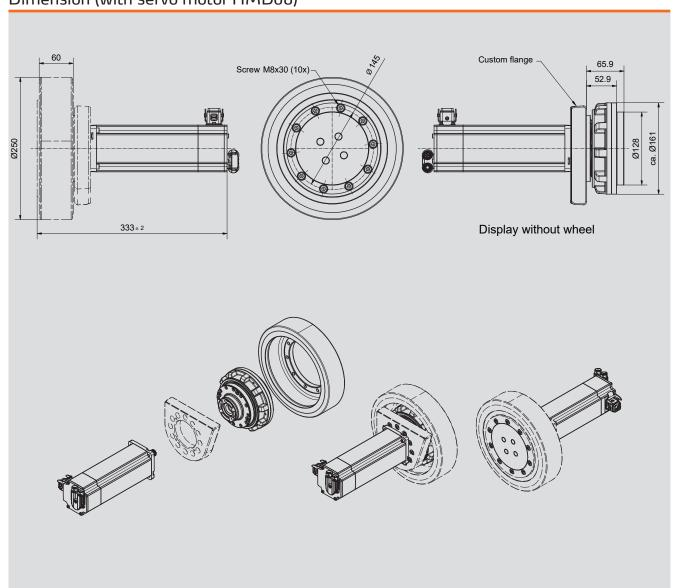
HeiMotion with reinforced planetary gear with direct mounting
